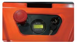
Battery deep discharge protection device, voltage discharge indicator with low voltage automatic cutting and lifting function, for higher battery lifetime. Proofed emergency switch and voltage discharge indicator, make it more durable and reliable.
