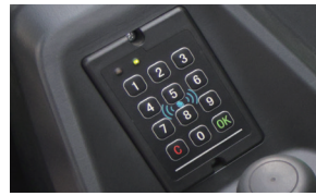
The multi-function password lock can manually enter the password or swipe the card to start, which simplifies the authorization operation process and meets the requirements of multi-shift work.
