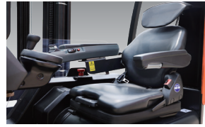
Suspension seat The highly elastic shock-absorbing seat greatly reduces the transmission of vibration to the driver. At the same time, the combination of the automotive-grade bionic curved backrest can effectively reduce the driver's driving fatigue; the seat can be adjusted in multiple positions to meet the operation of different heights and body shapes. user needs.
