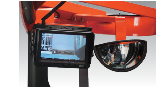
High-definition monitoring system, real-time monitoring of cargo stacking.
