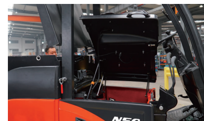
Fully openable cover design makes the maintenance of battery, motor, hydraulic piping, electronic controller and other parts extremely convenient and efficient.
