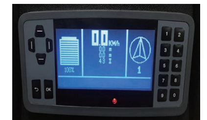
Standard angle sensor enables real time observation of steering wheel angle, along with speed reduction automatic deceleration while turning.
