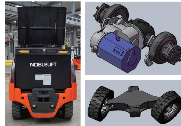
Transmission system: horizontal fan-shaped drive axle mounted in parallel, large transmission ratio. The battery is located at the bottom of the chassis which ensures great stability of the forklift. Hydraulic system: low noise gear pump with fully hydraulic power steering. Low noise and comfortable operation.
