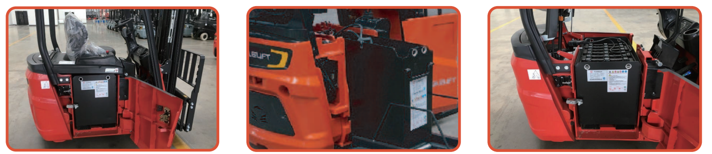
■ Battery compartment with fork pockets for 16N
