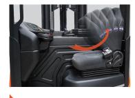
The high suspension seat greatly reduces the vibration transmission to the driver. At the same time with the automobile-type bionic curved backrest, it can effectively reduce the driver's driving fatigue. The seat can be adjusted to meet the needs of operators of different heights and shapes.
