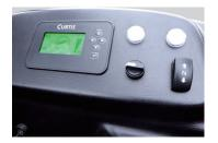
The multi-function color LCD instrument can display the steering wheel position, battery power, power alarm, fault code, working time and driving speed and other information.
